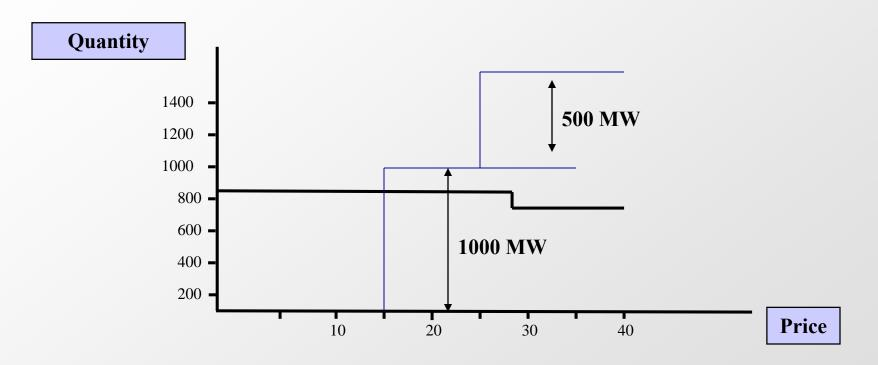
Unit 2: max 1000 MW, 15 Euro/ MWh
